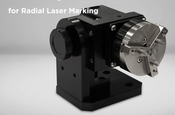
The D65 is a robust, compact rotary axis ideal for 360° radial laser marking. D65 can be used with any of our systems, but is ideal in our compact Minilase product line. The unit features a manual three jaw holding chuck along with multi-diameter fingers for holding the ID or OD of components. A tilting features enables marking on complex angles or inner diameters. When sold independent of a laser workstation, the D65 is supplied with a driver and power supply expansion box.
